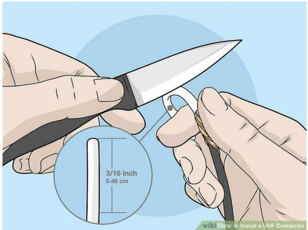
Cut the inner insulation about  $\frac{3}{16}$  inch (0.48 cm) from the cable's end. Folding back the braided threads will expose the inner dielectric insulation that surrounds the center metal conductor. You'll need to be even more careful cutting this than you were when you stripped the outer jacket. Slice only the thin polyfoam insulation without nicking the center conductor.
