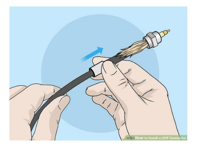
**Slide the ferrule to the base of the connector and crimp it.** Once you've crimped or soldered the center pin and conductor tip, you can crimp the ferrule to the back of the connector housing. Slide the ferrule over any exposed braided threads and over the the back side of the connector. When it's flush, insert it into the jaws of the crimping tool and squeeze the tool to fasten the ferrule to the connector housing.
