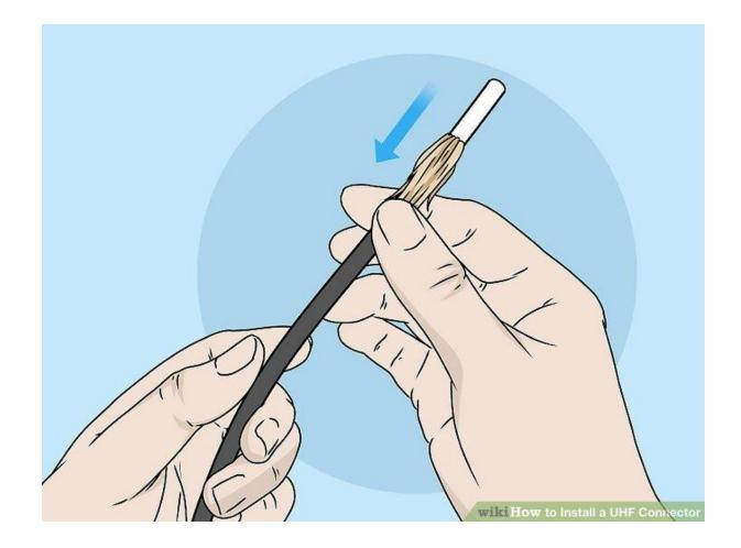
**Fold back the braided shield.** After you've cut the end of the cable, you'll see fine, braided threads surrounding the foil that encases the inner conductor. Fold these threads back from the inner casing and wrap them clockwise around the cable.
