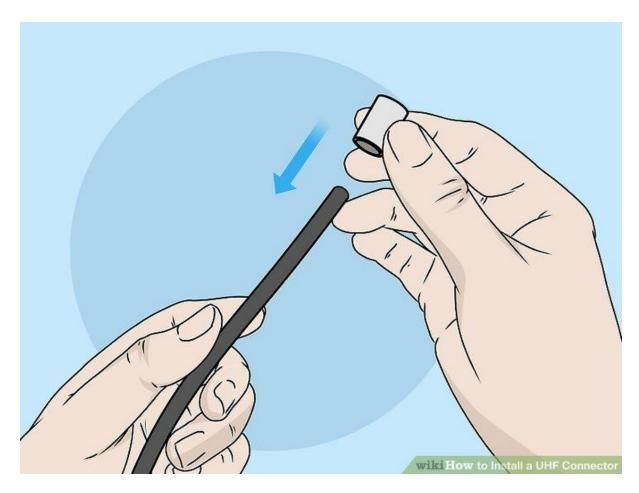
**Slide the crimping ferrule over the cable's outer jacket.** Start by inserting your cable through the crimping ferrule. Typically, a UHF connector set includes the connector housing itself and a crimping ferrule, which is a metal cylinder that helps secure the connector to the cable.
